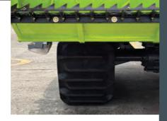
★ Cutter position is well beyond track system for cutting near ridges
